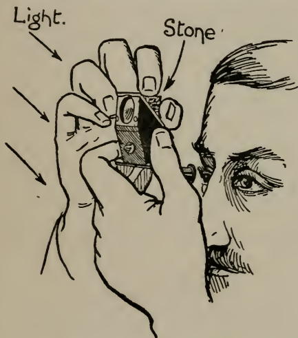
FIG. 17.—Method of Using the Refractometer.
